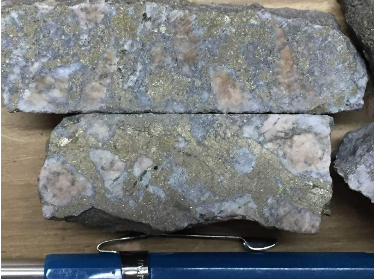
Figure 7-16 Hydrothermal Breccia: Intergrown Chalcopyrite-pyrite as Matrix to Sub-rounded Clasts of Potassic-altered Intrusive Rock, Pass Zone, hole 53 centered at 70.0m
