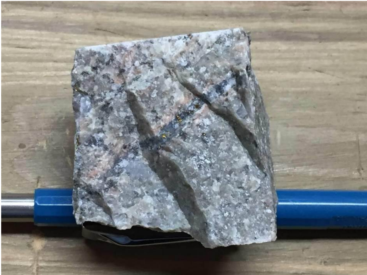
Figure 7-17: Close-up of Core Displaying Two Orientations (parallel to core axis and at 30° to core axis) of Quartz-chalcopyrite+/-molybdenite veinlets (with potassic halo), East Zone, DDH 107 at 194.2m (Lane, 2019)
